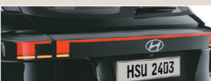
LED rear turn signal with sequential function
